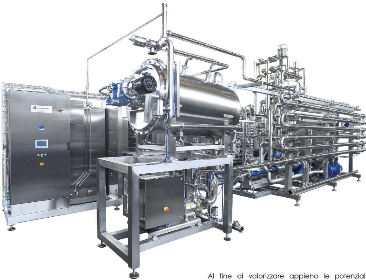
OHMIC ASEPTIC PLANT FOR PESTOS AND SAUCES
