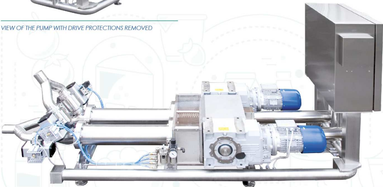
VIEW OF THE PUMP BODY WITH PROTECTIONS REMOVED
