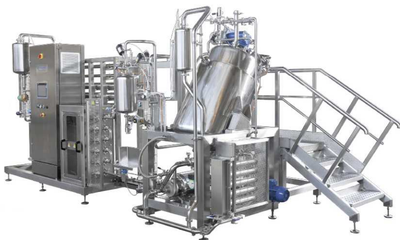
PILOT ASEPTIC OHMIC PLANT FOR VEGETABLE PUREES WITH AND WITHOUT SOLIDS
