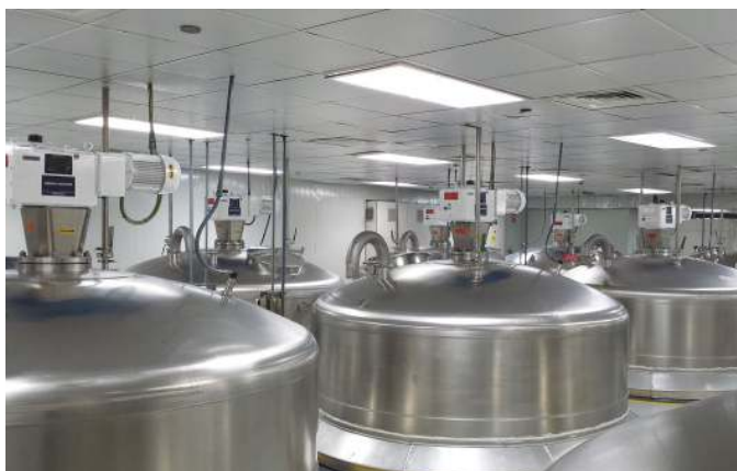
Chemineer HT agitators used in a sanitary environment mixing a consumer product
