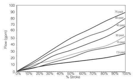
% STROKE VS FLOW (2" MK96A – JORLON DIAPHRAGM – 19 CV)
